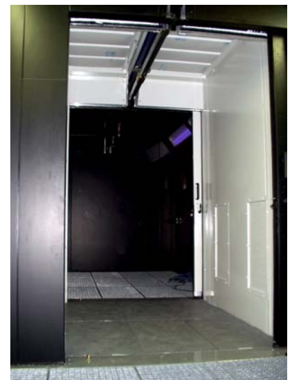
Séchage ressuage aéronautique Aeronautic penetrant testing drying
